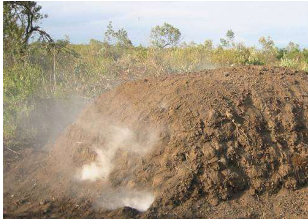
Charcoal kiln in the early stages of firing, Narok, Kenya. Source: Rob Bailis & Dan Kammen
