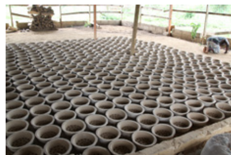
Clay stove liners waiting to be fired.
