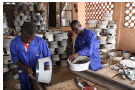
Making stove bodies in the production centre near Accra.
