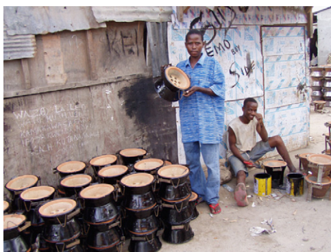
Fig. 2. Charcoal stove (Kenyan Jiko), made of clay/metal, artisanal production, Kenya (Photo: Marlis Kees, GTZ).
