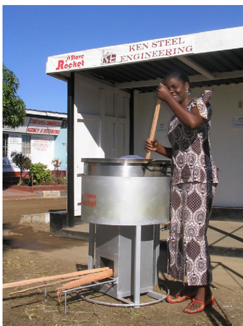
Fig. 3. Wood stove (Institutional Rocket Stove), made of metal and insulation material, artisanal production, Malawi (Photo: Andreas Michel, GTZ).
