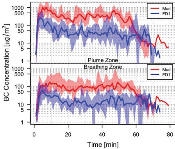
**Figure 1.** Time series data for (upper) plume zone and (lower) breathing zone BC concentrations during cooking. Dark lines show median values, with shaded regions indicating minimum and maximum values from repeated tests.
