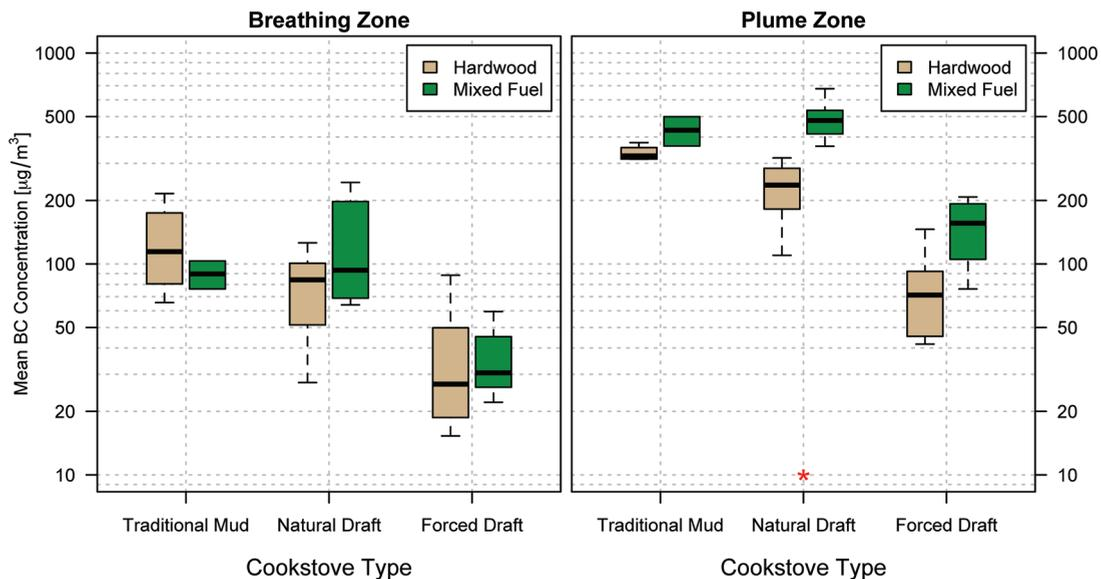
**Figure 3.** Comparison of BC concentrations for hardwood and mixed fuel tests in (left) the breathing zone, and (right) the plume zone. In this plot, a red star under the boxes means that the mean values for hardwood and mixed fuel tests are statistically different for that stove technology class (at the 95% confidence level,  $p < 0.05$ ).
