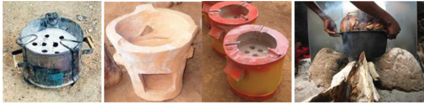
Fig. 1. Charcoal stoves ( left, metal; center left and center right, ceramic ), and three-stone fire stove ( right ).
