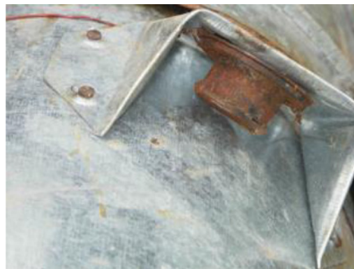
Fig. 2. iButton attached to the inside of the handle of a top-lit updraft in Uganda.
